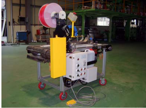
Fig. 10. Picture of the prototype of the automatic bundling machine.
